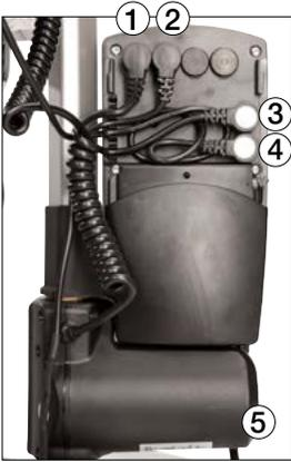
Remove the control box cover to make the connections as described below. Use a screwdriver or similar; refer to the special labels on the control box.
