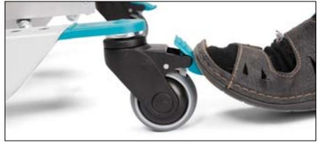
Bure Double is fitted with braked castors with directional locking (green pedal). Depress the foot brake to set it and lock the castor. To unlock, press down on the protruding part of the brake. Locking affects rolling and swiveling.
